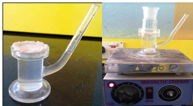
Fig 4. Franz Diffusion set up for drug release (with mice skin and dual patch)
