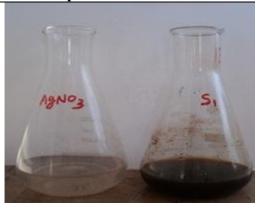
AgNO 3 = 1mM AgNO 3 without extract. AgNPs (S1)=1 mM AgNO 3 with A.aspera extract after 5 h of incubation (Brown colour).
