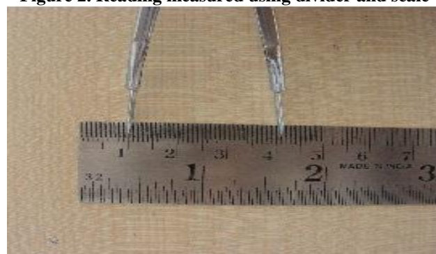
Figure 2. Reading measured using divider and scale
